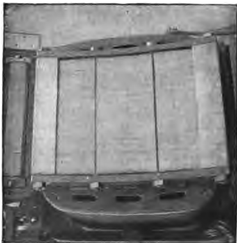
FIG. 297. The pole face of a synchronous motor showing the damping grid, which is used to prevent hunting. The General Electric Co.
